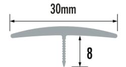
**TDY 50** Self Adhesive or Pre-drilled Threshold Profiles Laminate, parquet, carpet, pvc flooring, ceramic
