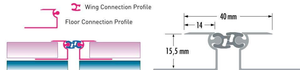
**TDL 20** Ceramic perforated Under-floor Expansion Jointing Profiles
