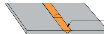
The welding rod is placed in the chamfer between two floor coverings. When heated, it melts and fills the entire space to ensure complete watertight seal.
