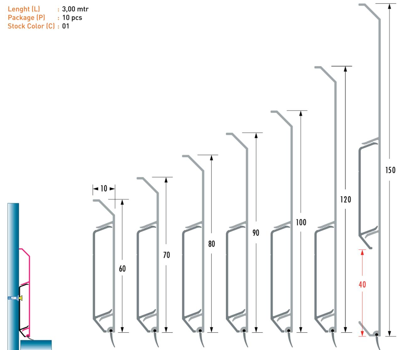
**TSA** Ceramic perforated Under-floor Ceramics Finish and Outer Corner Profiles
