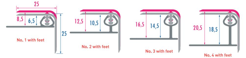
**TSI** Ceramic perforated Wide sided Ceramics Inner Corner Profiles
