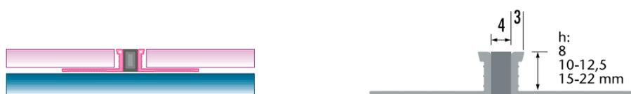
**TFL 10** Ceramic perforated Ceramic Movement Control Profiles
