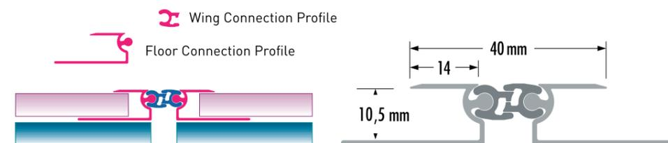
**TDL 10** Under-floor Expansion Jointing Profiles
