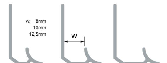
**TFL 03** Ceramic perforated PVC Flooring - Linoleum Under - Floor Expansion Jointing Profiles
