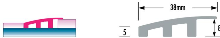
**TKFL 37** Self Adhesive or Pre-drilled Threshold Profiles
