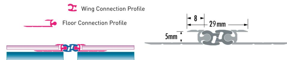
**TDL 10** Under-floor Expansion Jointing Profiles
