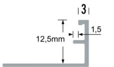
**TSD** Ceramic perforated Wide sided Ceramics Outer Corner Profiles
