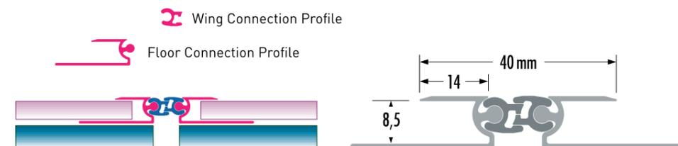
**TDL 10** Under-floor Expansion Jointing Profiles
