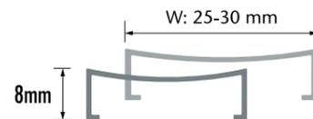
**TFN** Ceramic perforated Right Angled Narrow-edge Ceramic Finish and Corner Profiles
