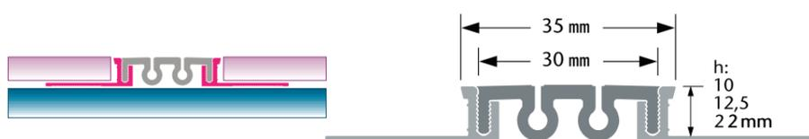
**TFL 06** Ceramic perforated Ceramic Movement Control Profiles
