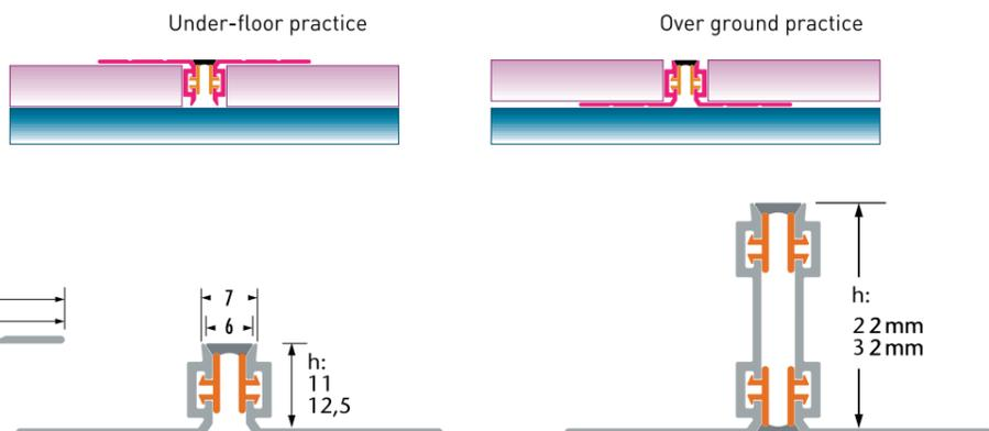
**TDL 10** Ceramic perforated Under-floor Expansion Jointing Profiles
