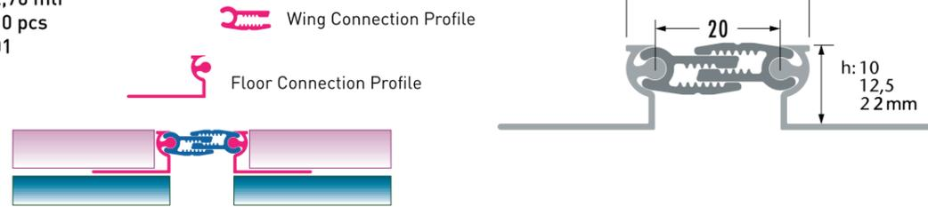
**TDL 30** Ceramic perforated Under-floor Expansion Jointing Profiles
