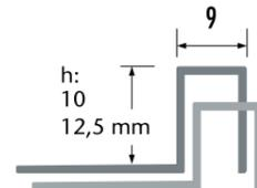
**TKO** Ceramic perforated Right angle wide edge ceramic finish and corner profile
