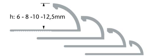
**TSAG** Ceramic perforated Under-floor Ceramics Finish and Outer Corner Profiles
