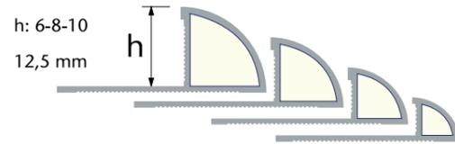
**TKR 10** Ceramic perforated Under-floor Ceramics Finish Level Difference Profiles
